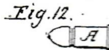
Figure 1. The non-specified caliber rimfire cartridge depicted as Figure 12, on Henry’s 1860 patent No. 30446, for “improvement in magazine firearms.” The description reads, “Fig. 12 represents the ammunition used – a conical or round ball inserted in a metal cartridge. A. having a hollow flange round the base, containing a priming of fulminating powder” (McDowell 1984: 65-66).
